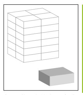
Storage conditions: cool and dry place, away from direct sunlight and at room temperature. Between -20 °C e -30 °C the material becomes fragile. Handle with care to avoid breakage and shattering.
